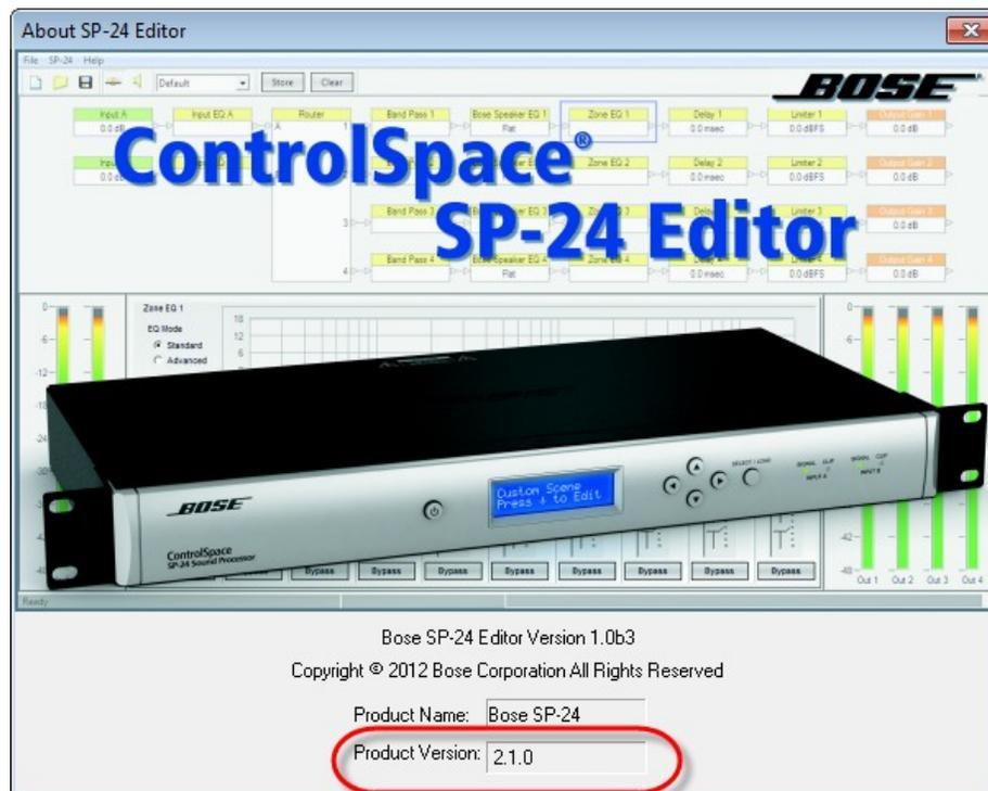
Fig. 6.1- About SP-24 Editor Dialog, firmware version is shown in lower section
