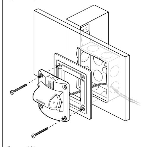
Do not overtighten. If using a power drill, set to a low torque setting.
