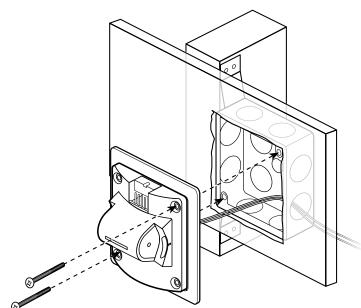
Do not overtighten. If using a power drill, set to a low torque setting.
